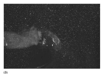
Fig. 6 Gas entrainment in a single discharging bottom branch, PIV image in (a) vertical and (b) horizontal planes
