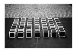
Fig. 2 USEPA Meteorological Wind Tunnel: 3D Array of Buildings (courtesy of Michael Brown, LANL). Previous reported studies used the USEPA wind-tunnel data to test flow simulation models but did not address their effects on CT.
